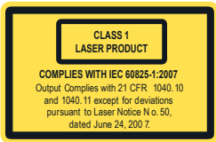
Figure 3. FDA (CDRH) warning label (Class 1)
