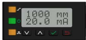
Figure 11. LE550 Display in Run Mode
