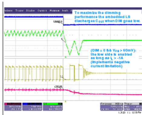
Figure 28. LED current falling edge
