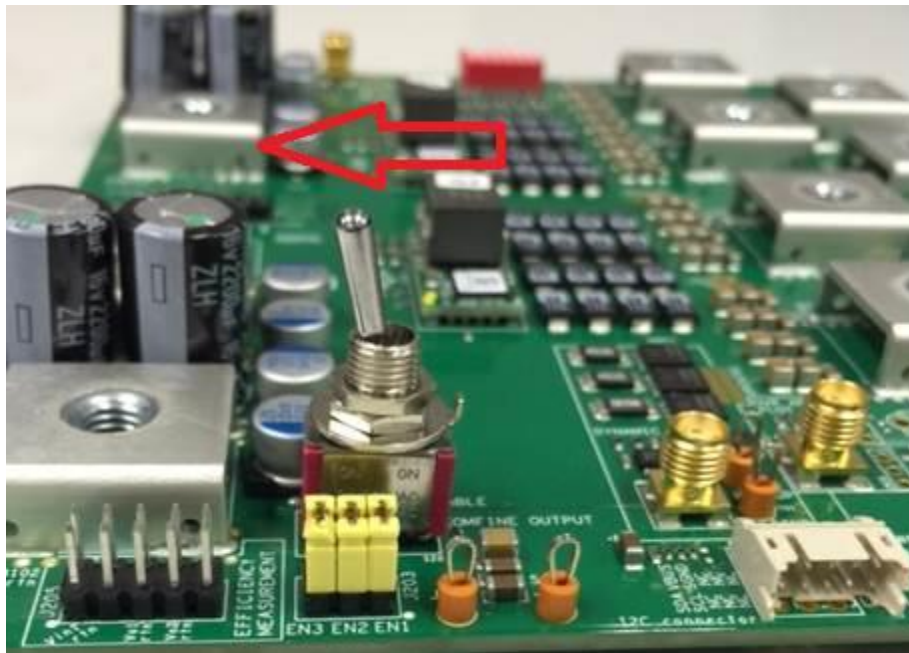
Fig. 7 – Toggle switch position to enable the outputs of the modules
