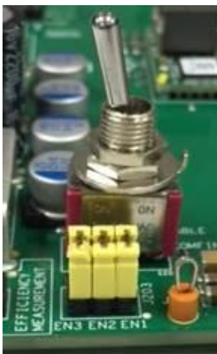
Fig. 4 – Enable jumper location and population
