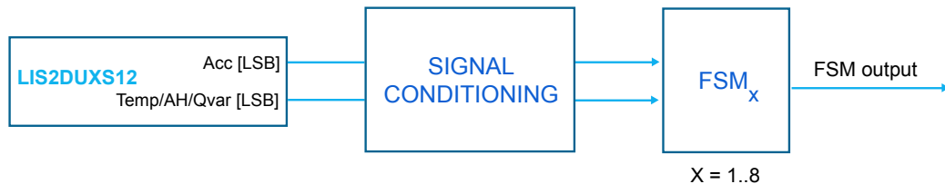
Figure 11. State machine in the LIS2DUXS12
