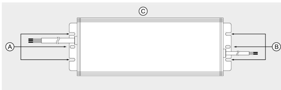
Fig. 3 Mounting Hole Locations
