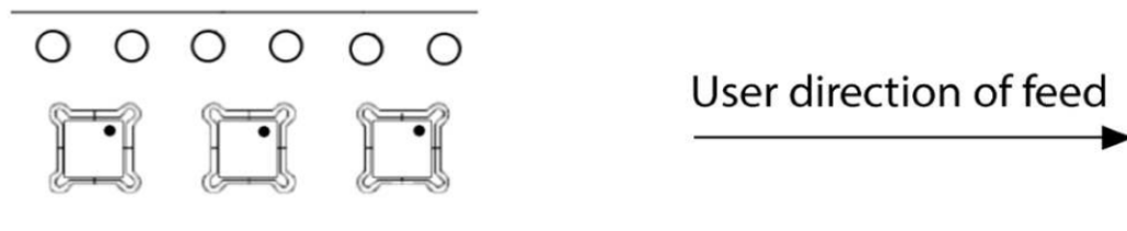
Figure 29. Package orientation in carrier tape
