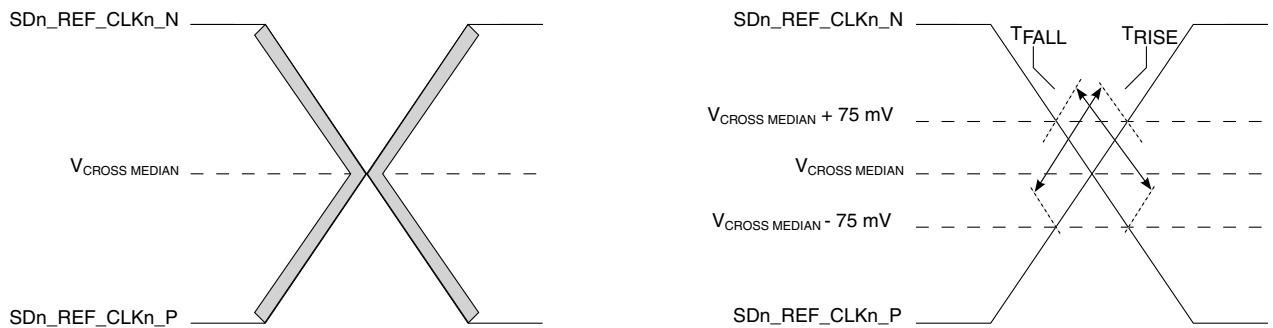
Figure 84. Single-ended measurement points for rise and fall time matching
