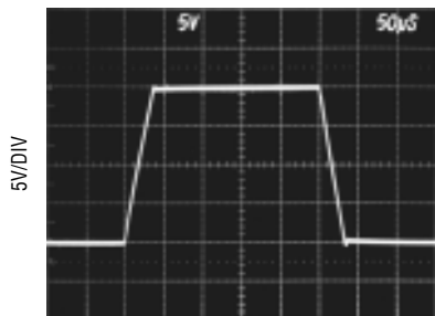
Large-Signal Transient Response
