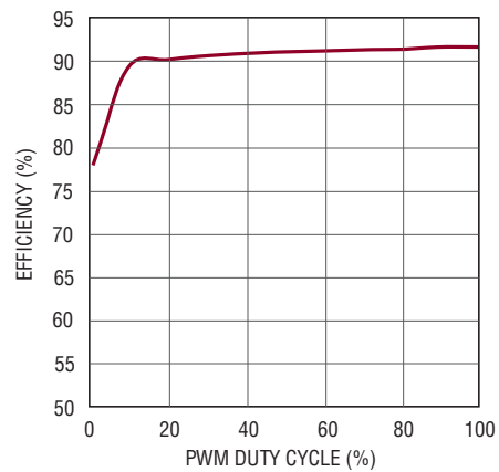
Efficiency vs PWM Duty Cycle for 200mA LEDs
