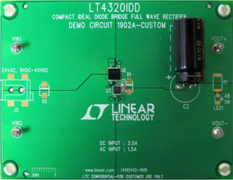
Figure 4. Demonstration Circuit 1902A Used in Figure 3 Thermograph
