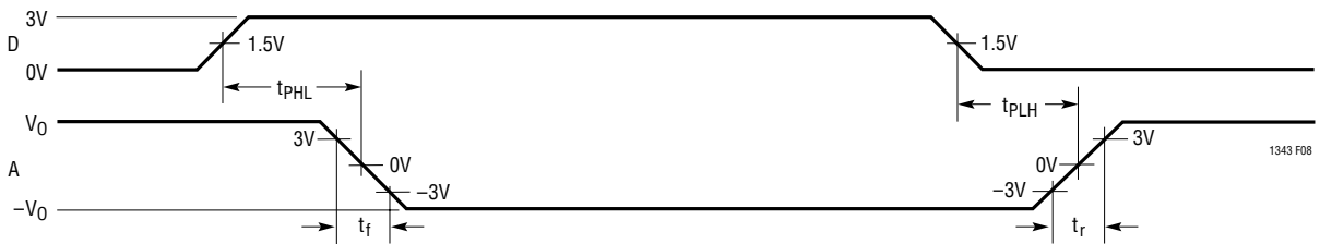
Figure 8. V.10, V.28 Driver Propagation Delays
