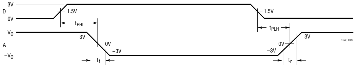
Figure 8. V.10, V.28 Driver Propagation Delays
