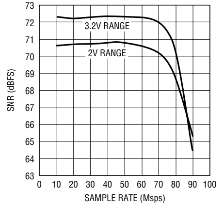
SNR vs Sample Rate, Input Frequency = 5MHz, -1dB
