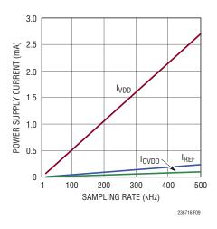
Figure 9. Power Supply Current of the LTC2367-16 Versus Sampling Rate
