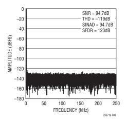
Figure 8. 32k Point FFT with f<sub>IN</sub> = 2kHz of the LTC2367-16
