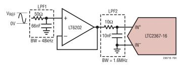
Figure 4. Input Signal Chain
