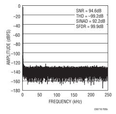
Figure 5b. 32k Point FFT Plot with  $f_{\text{IN}}$  = 2kHz for Circuit Shown in Figure 5a
