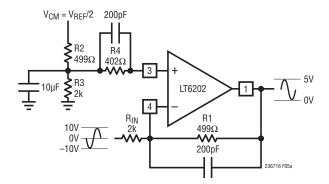
Figure 5a. LT6202 Converting a ±10V Bipolar Signal to a OV to 5V Input Signal
