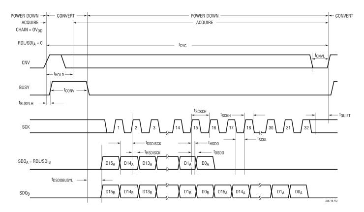
Figure 12. Chain Mode Timing Diagram
