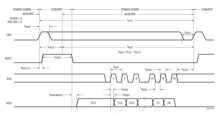
Figure 10. Using a Single LTC2367-16 in Normal Mode
