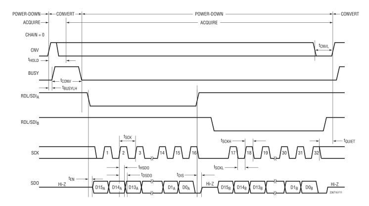
Figure 11. Normal Mode With Multiple Devices Sharing CNV, SCK and SDO
