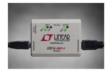
speed selection configures integrated pull-up resistors on the upstream port to match those sensed on the downstream device. By default, downstream devices are powered (up to 1W) by the upstream bus through an isolated DC/ DC converter. Optionally, a wall adapter can be used, increasing available power to downstream devices to 2.5W.
