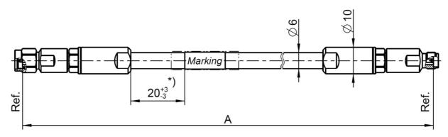
All dimensions are in mm; tolerances:  $\pm$  3mm for A  $\leq$  300 mm;  $\pm$  1% for A > 300 mm \*) If length "A" < 150 mm marking is mount centric ±5 mm
