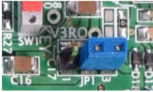
Figure 12. Jumper Switch JP1
