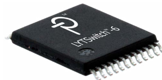
Figure 2. High Creepage, Safety-Compliant InSOP-24D Package.
