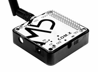
The module base has a DC power input interface. Please strictly follow the input range (5-12V) to prevent damage to the module when using this interface to connect to the power supply. The internal power DIP switch can adjust the voltage level of the internal terminal VIN to adapt to different modules.
