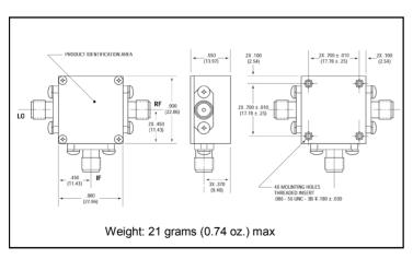
\* Dimensions are inches (millimeters)  $\pm 0.015$  (0.38) unless otherwise specified.
