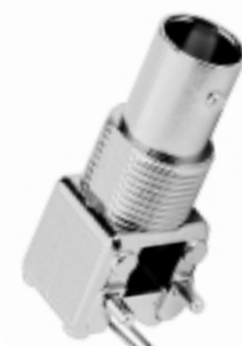
Metal Housing 31-71042 (Round Pins)
