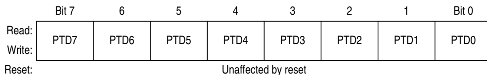
Figure 11-13. Port D Data Register (PTD)
