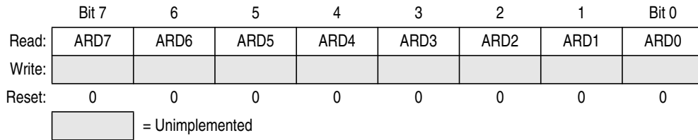
Figure 13-19. ESCI Arbiter Data Register (SCIADAT)
