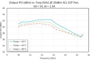
Output IP3 (dBm) vs. Freq (GHz) @ 25dBm SCL O/P Pwr, Vd = 5V, Id = 1.3A
