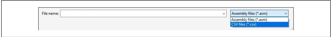
Figure 20. Select the “CSV files” option in the bottom right hand corner of the file viewer window to display the csv files.
