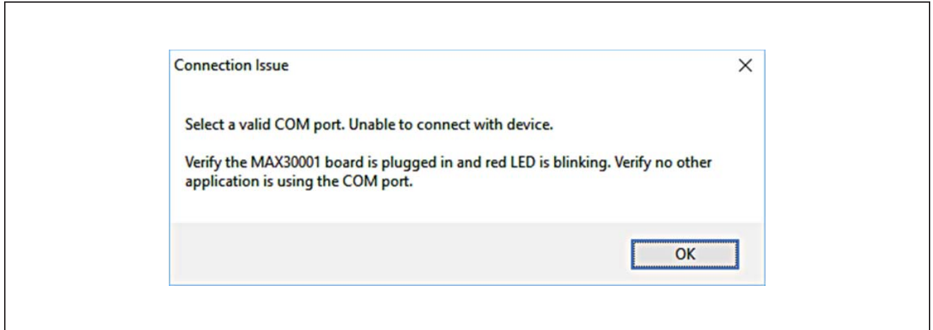
Figure 1. The Connection Issue Dialog Box Appears If The GUI Does Not Detect the EV Kit.
