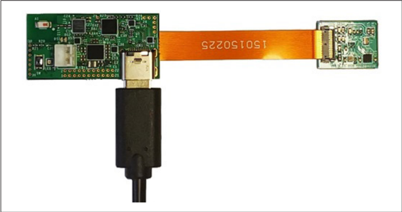
Figure 8. Hardware Setup (MAXM86146 EV System Micro PCB)
