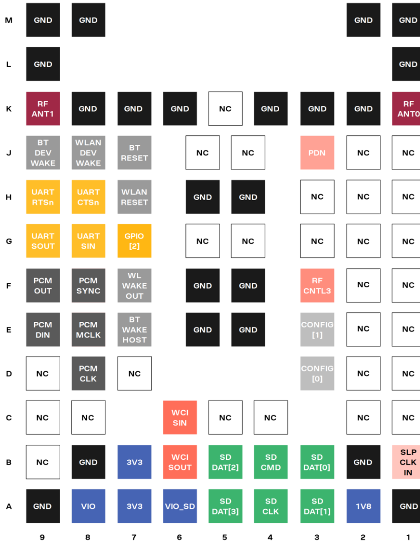
Figure 14: MAYA-W1 series pin assignment (top view)
