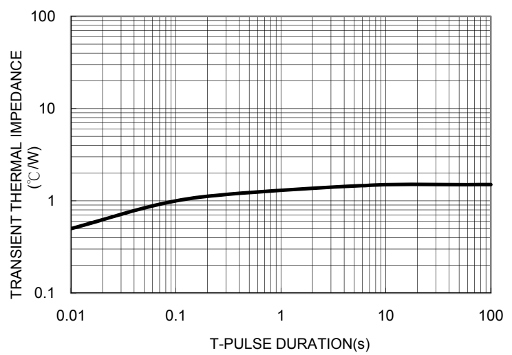
FIG. 6 TYPICAL TRANSIENT THERMAL IMPEDANCE
