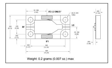
\*For base model, only the IF1 port is connected. For the "-2" model, only the IF2 port is connected.
