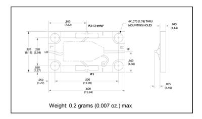
\*For the base model, only the IF1 port is connected. For the "-2" model, only the IF2 port is connected.
