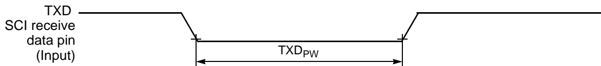
Figure 10-16 TXD Pulse Width
