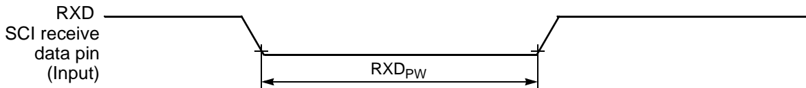
Figure 10-15 RXD Pulse Width
