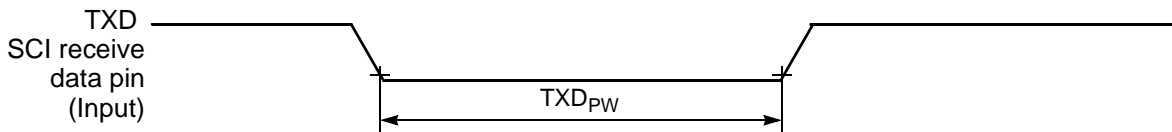
Figure 10-16 TXD Pulse Width
