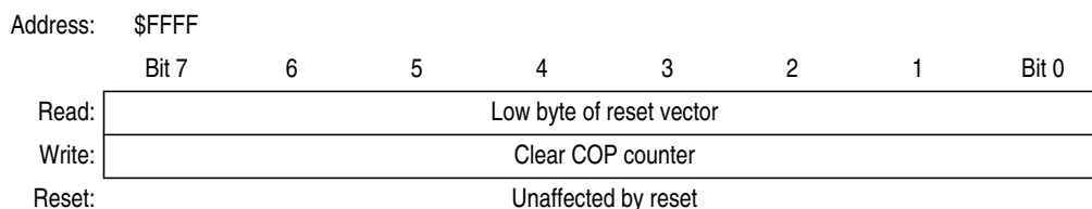
Figure 19-3. COP Control Register (COPCTL)
