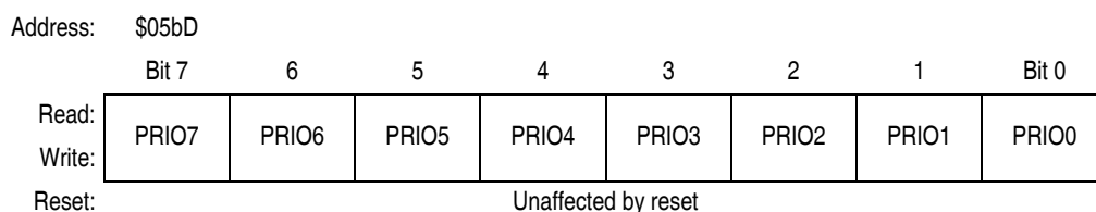
Figure 12-14. Transmit Buffer Priority Register (TBPR)
