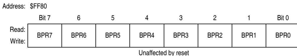
Figure 2-4. FLASH-1 Block Protect Register (FL1BPR)
