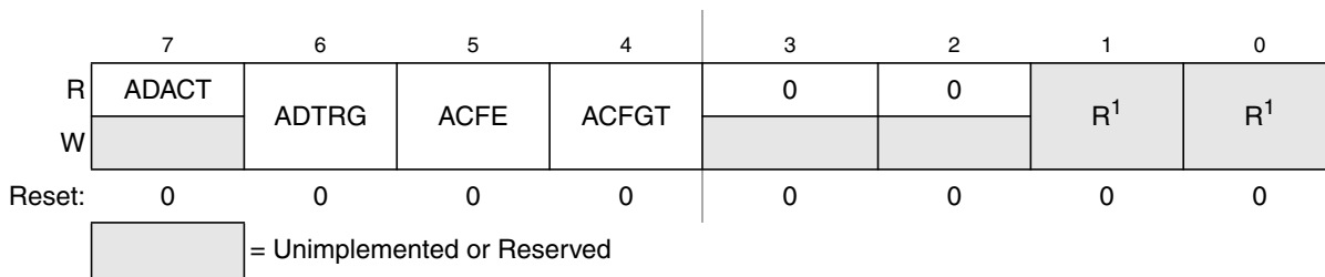
Figure 14-5. Status and Control Register 2 (ADC1SC2)
