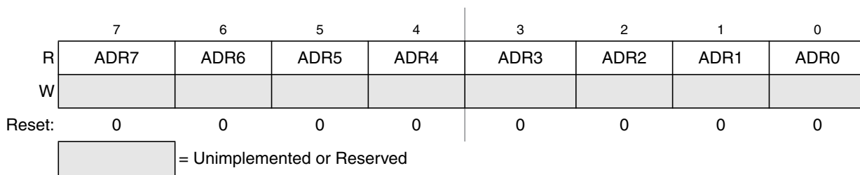
Figure 14-7. Data Result Low Register (ADC1RL)
