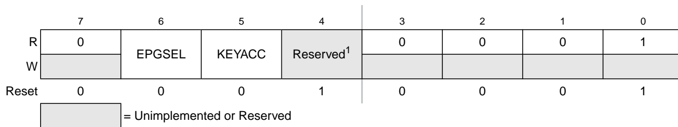
Figure 4-7. Flash Configuration Register (FCNFG)
