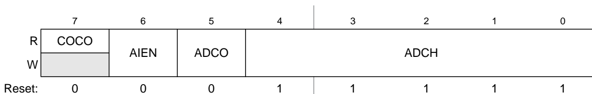
Figure 10-3. Status and Control Register (ADCSC1)
