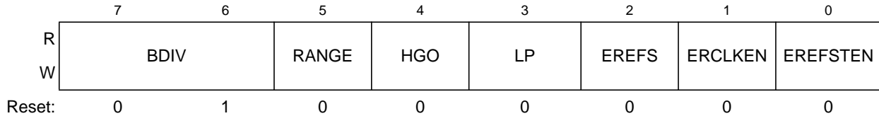
Figure 8-4. MCG Control Register 2 (MCGC2)
