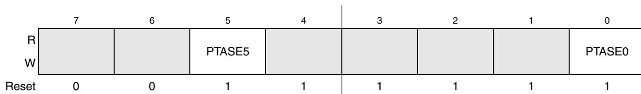
Figure 6-5. Output Slew Rate Control Enable for Port A (PTASE)
