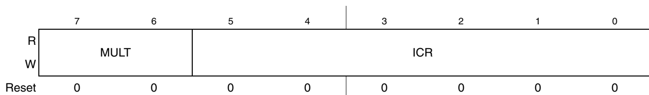
Figure 11-4. IIC Frequency Divider Register (IICF)
