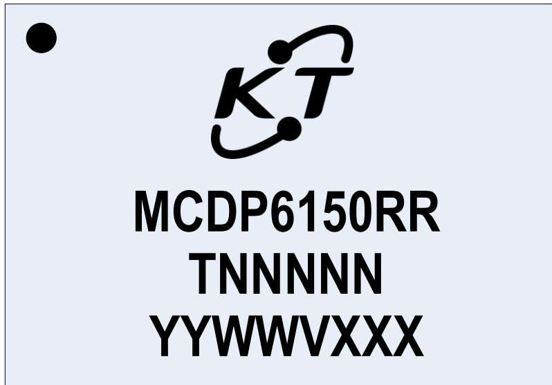
Figure 19. MCDP6150 Ex-VQFN46 Marking Template
