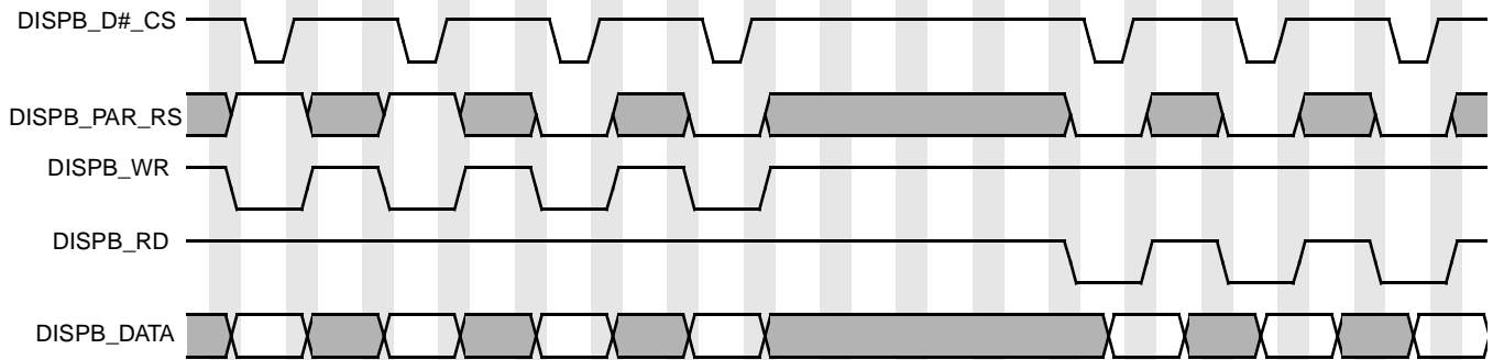
Single access mode (all control signals are not active for one display interface clock after each display access)
