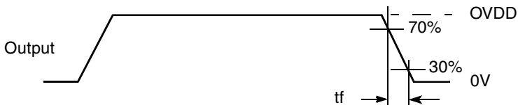
Figure 7. Definition of Timing for Standard and Fast-Mode
