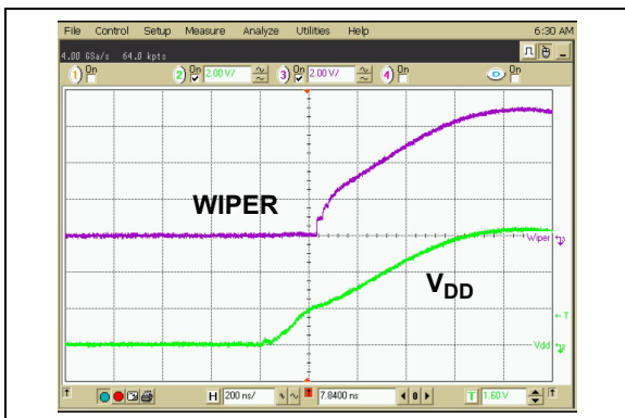
FIGURE 2-15: 2.1 k \Omega – Power-Up Wiper Response Time.
