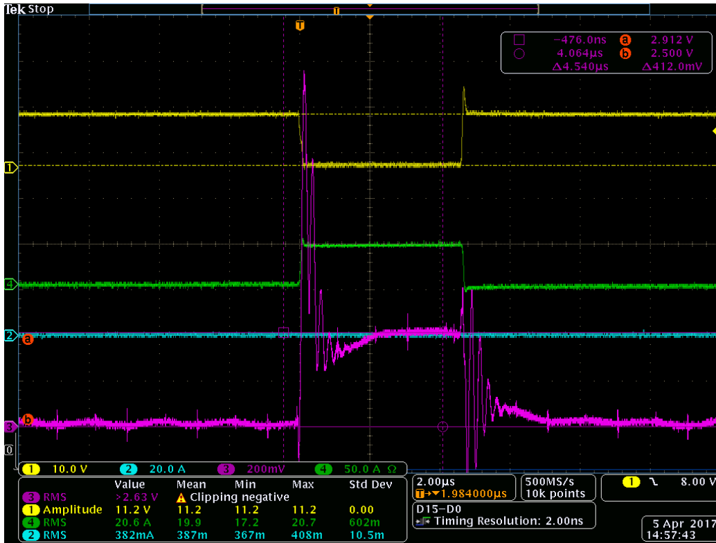
Figure 18. Noise on a Shunt Resistor with Wrong Input Impedance
