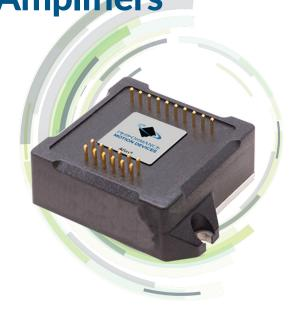
**ATLAS® Digital Amplifiers** are compact single-axis amplifiers that provide high performance torque control for DC Brush, Brushless DC, and step motors. They are packaged in a compact, solderable module and are ideal for use in positioning motion control, velocity control, and precision force control applications.
