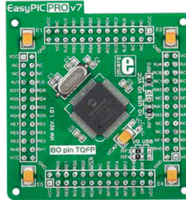
3 Figure 4-7: Standard 80-pin MCU card with PIC18F8722 .
