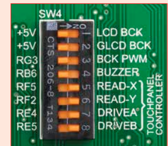
Figure 14-5: Turn on switches 5 through 8 on SW4 to enable Touch panel controller
