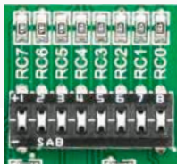
Figure 6-2: Tri-state DIP switch on PORTC
