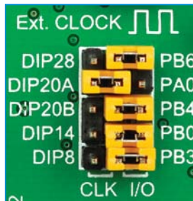
Figure 4-7: Position of the jumpers for DIP20A
